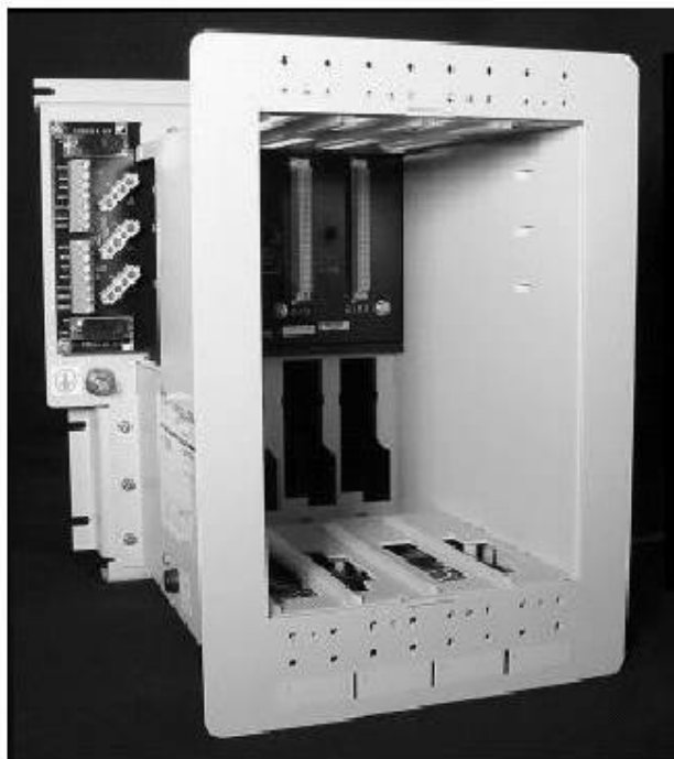
Remote I/O Rack Figure 4-6
