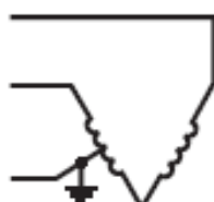
(h) Three-phase open delta; Four-wire: Earthed mid point of one phase
