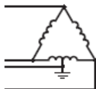
(g) Three-phase delta; Four-wire: Earthed mid point of one phase
