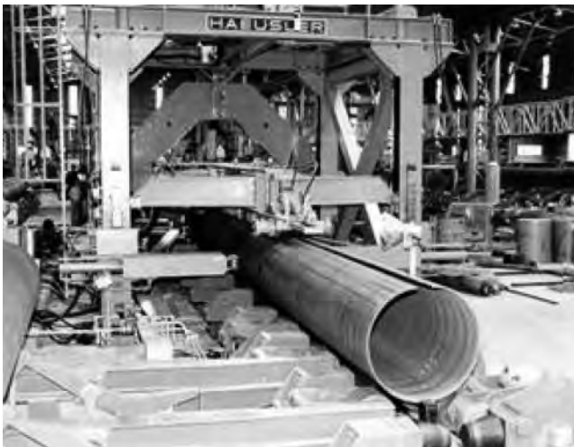
Figure 11.14 Pipe welding machine.
