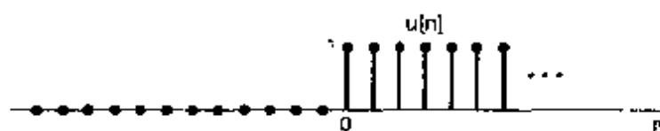
Figure 1.29 Discrete-time unit step sequence.
