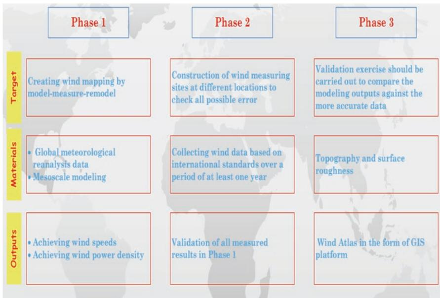
Fig. 1.5 The required phases for the wind energy assessment
