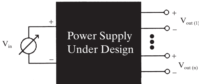
Figure 3-17 The SMPS treated like a black box.
