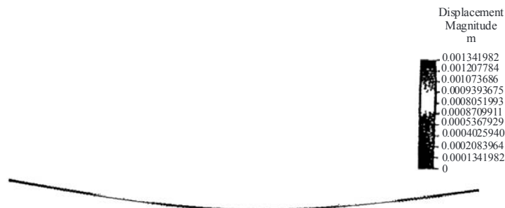
Figure 1: 400mm beam deflection with shear area included
