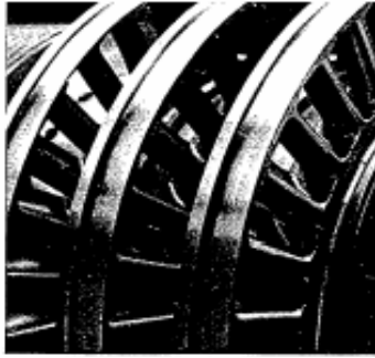
Rotor drum stage blading with integral shrouding
