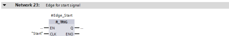
Fig. 8.29 Example of edge evaluation with EN/ENO box in the function block diagram
